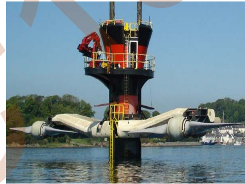
Figure 3 : SeaGen horizontal axis turbine with pitch variation system
