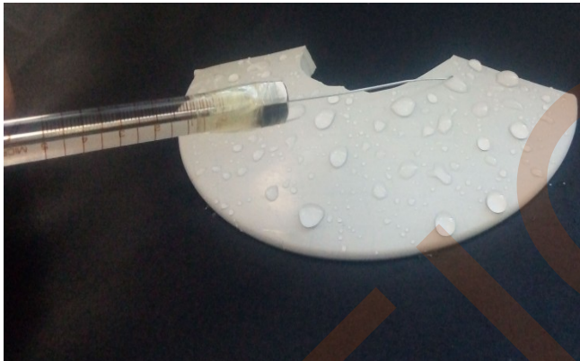
Fig. 2. Measuring the volume of drops of natural rainwater using a microliter graduated syringe
