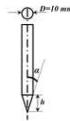
Figure 2. Scheme of the corona electrode
