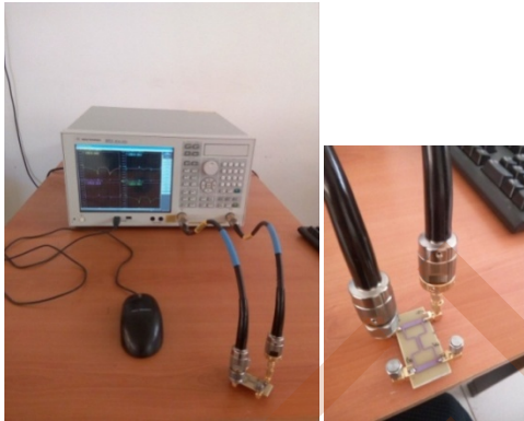
Figure 4. (left) Measurement setup: a network analyzer E5071C being used for S -parameter measurement, (right) component under test.
