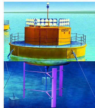
Figure 4: KOBOLD vertical axis turbine with floating platform
