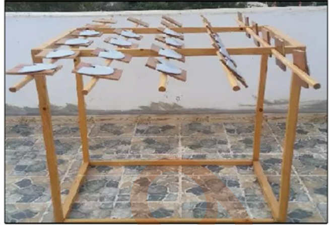
Fig. 3. Stem's device ensuring the variation of inclination of the angle \alpha of the silicone insulation in compararaison to the horizontal
