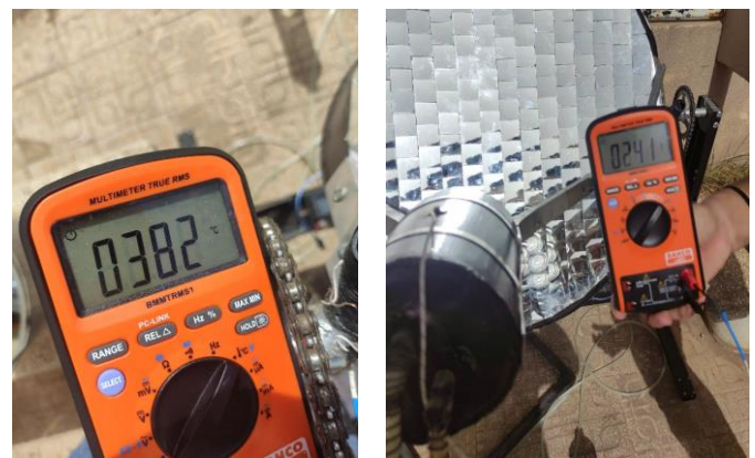
Fig. 9 Temperature on the surface and inside the absorber
