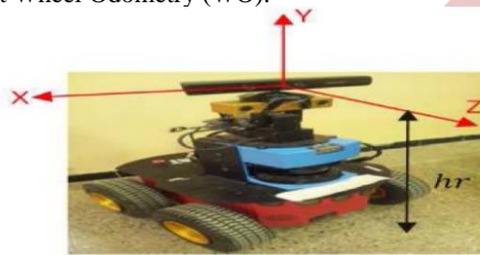
Figure.14 The mobile robot Pioneer with a Kinect Camera.
