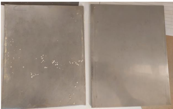
Figure 8. the collected plates for an applied positive voltage 14kV
