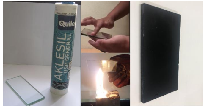
Figure 1. Essential steps in the manufacture of a superhydrophobic coating on a glass plate.
