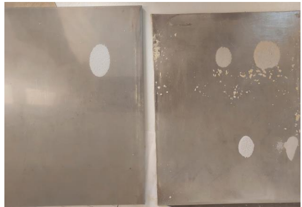
Figure 10. The collected plates for an applied positive voltage 17kV
