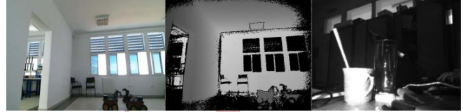
Figure.2. Kinect provided data: RGB image (left), DEPTH (middle) and infrared image (right).
