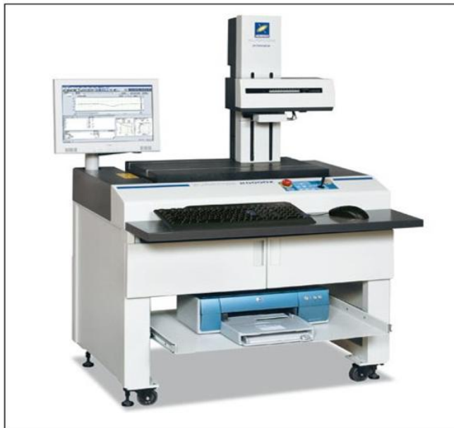
Figure 3. Photo of a profilometer from the HV laboratory in Zittau (Germany)
