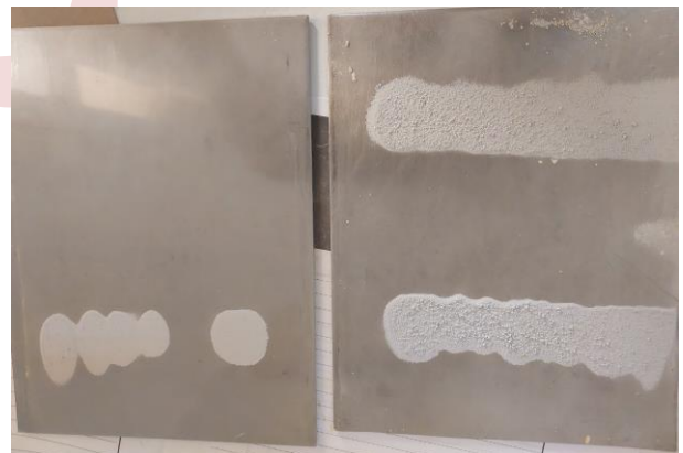
Figure 12. The collected plates for an applied positive voltage 20kV
