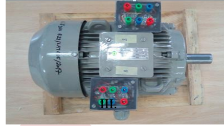
Figure 1. Photo of a Double Stator Induction Machine
